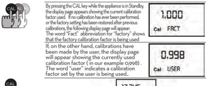
The flow chart alongside shows the switchover logic from one display page to another. In this condition, the Reset key permits switching from User factor to Factory factor.
